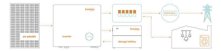
PV stands for 'photo-voltaic' - it means converting light into electricity.
